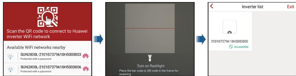
Figure 7-6 Scanning the QR code to connect the mobile phone to the SUN2000L directly
