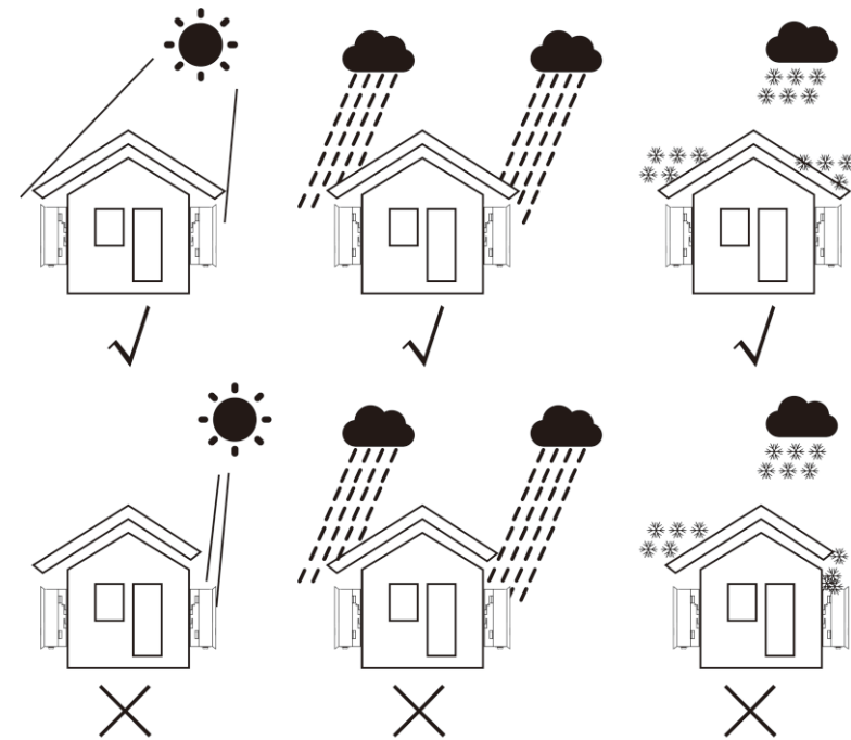
Figure 4.1 Recommended Installation locations
